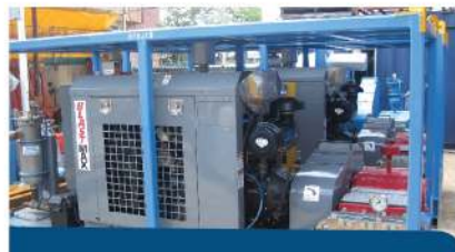
AQUA DYNE GA 200 SERIES RATED 8.57 GPM AT 40,00 PSI
